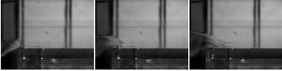
FIGURE 9. Initial stages of water shipping: example characterized by rather small spatial scales. The surface tension rounds the water front entering the deck so that the cavity formation is practically prevented. Time increases from left to right with time interval of 0.04 s. Nominal regular waves: \lambda/f = 40 , H/\lambda = 0.06 .
