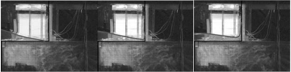
FIGURE 17. First stages of water impact with a vertical wall at 0.2275 m from the bow: global view. Numerical free surfaces (solid lines) are superimposed to the experimental video images. In the numerics, the initial plunging phase has not been modelled. Time increases from left to right with a time interval of 0.04 s. In the numerics, the time instants are \Delta t_{wod} = t - t_{wod} = 0.273, 0.313 and 0.353 s, with t_{wod} \simeq 7.89 s the instant of water-on-deck starting.
