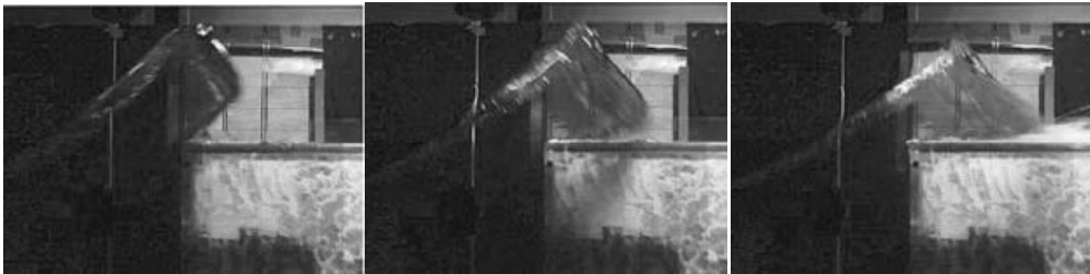
FIGURE 10. Initial stages of water shipping: example characterized by rather large spatial scales. The phenomenon starts as a large-scale plunging wave. The impact with the deck appears quite flat and involves a large area of the deck. The thickness of the deck is 11.8 mm. Time increases from left to right with time intervals 0.08 s and 0.04 s, respectively. Nominal regular waves: \lambda/f = 30 , H/\lambda = 0.08 .
