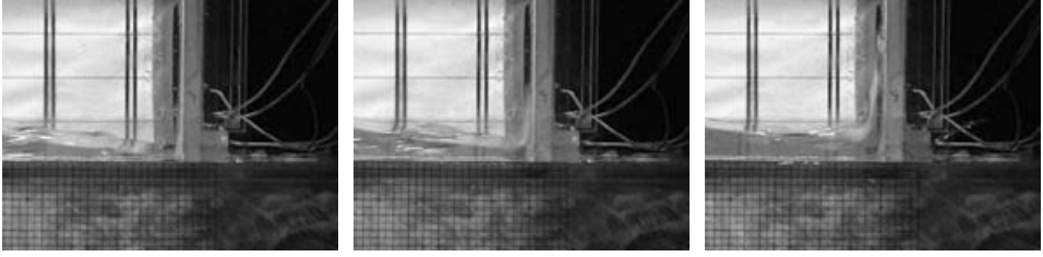
FIGURE 16. First stages of water impact with a vertical wall at 0.2275 m from the bow: enlarged view. The incoming water front can be approximated as a half-wedge. The impact causes a jet rising along the structure. Time increases from left to right with time interval of 0.04 s. Nominal regular incoming waves: \lambda/f = 40 , H/\lambda = 0.08 .
