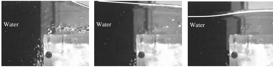
FIGURE 14. Evolution of the flow field near the bow edge during the later phases of water shipping. Bubbles are visible, partially convected along the deck and partially involved in the water run-down in front of the bow. To help interpretation of the images, the water profiles have been marked with white curves. The thickness of the deck is 11.8 mm. The time increases from left to right with a time interval of 0.04 s. Nominal regular incoming waves: \lambda/f = 40 , H/\lambda = 0.08 .
